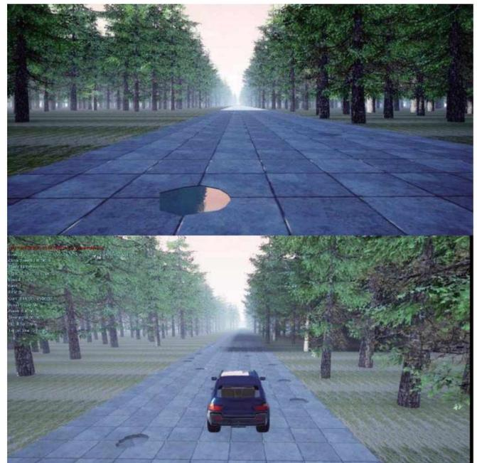
Fig. 1. Our virtual environment for learning pothole detection, which is based on AirSim [1] and VIVID [2].
